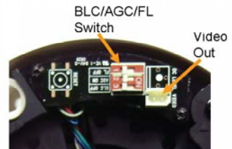
b. Camera control module for 270K, 410K pixel camera
