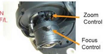
d. Control knobs for Varifocal Lens
